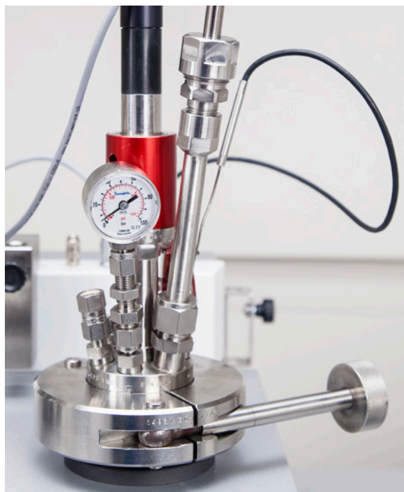
Figure 1. EasySampler probe in a pressure reactor
